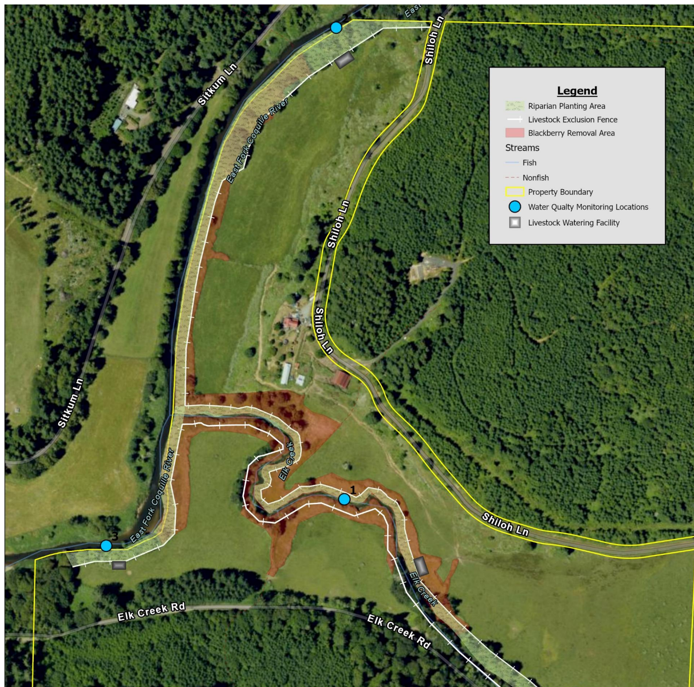
Figure 1. Map of the project area showing all the stages of the project. The objectives are to remove invasive blackberries along Elk Creek and the East Fork Coquille river, construct livestock exclusion fencing to prevent livestock from entering the waterways, and plant native species within the fenced riparian area.
